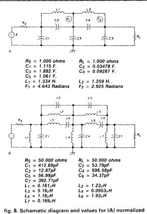
fig. 8. Schematic diagram and values for (A) normalized lowpass element, and (B) denormalized bandpass element of the bandpass filter.
